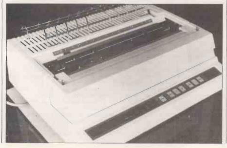
OUR FIRST impression on unpacking the NEC Spinwriter was one of superb production engineering. The case is the apparently now industry-standard cream colour well-cast in three metal parts which fit together perfectly. The front cover is articulated on long hinges which lift it clear of the tractor feed when fitted and it snaps shut again with reassuring firmness. Even the disposable security bolts which hold the machine during shipping are beautifully tooled.
